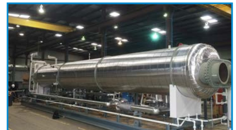
60 GPM Gas Sweetening and Hydrocarbon Dew Point Package, Pakistan
